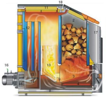
1. Chamber lid with extraction channel 2. Filling chamber with protective layer 3. Hot cast iron grate 4. Ashtray 5.Primary and secondary air motor 6. Secondary air 7.Primary air 8. Bottom air preheat 9. Secondary air nozzle 10. High temperature combustion chamber 11. Cleaning lid 12. Tubular heat exchanger 13. Dust extraction zone 14. Cleaning opening 15. Exhaust fan 16. Smoke sensor 17. Microprocessor control 18. Transport fitting
