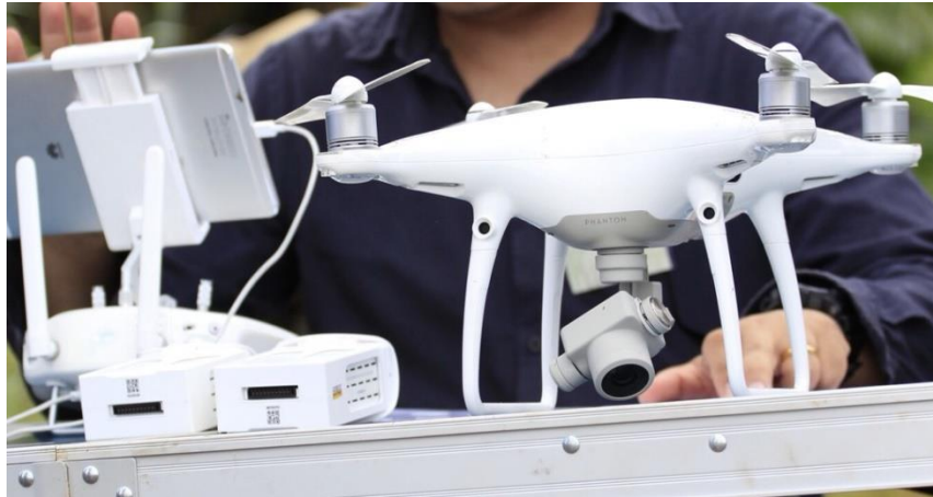
Figure 3 A drone owned by Forest Restoration Research Unit to be used for testing the prototype seed disperser system
